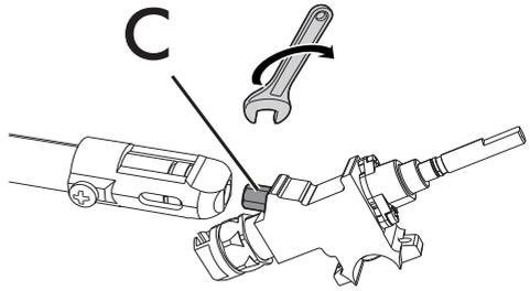
2. Use a spanner to remove the nozzles "C" and install the new ones for the required gas supply, following the indications given in the relevant table (see "Gas types and Countries").
