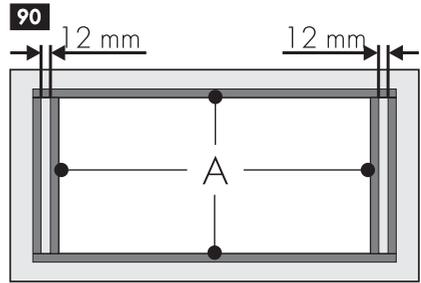
2. Use light pressure to make the seal stick to the edge around the hole cut in the worktop.
