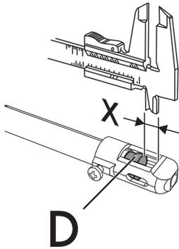
4. Move the Venturi tube "D" to adjust the air flow until distance "X" is reached as indicated in the paragraph (see Table "Burner and nozzle characteristics" - "Primary air adjustment (mm)") and then secure the tube by means of screw "A".
