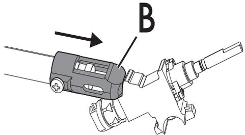
3. Reposition support "B" so that nozzle "C" is covered completely.
