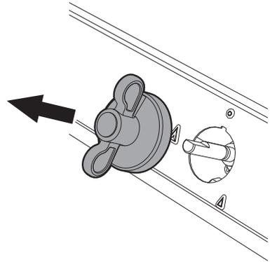
3. Remove the flame-spreader crowns and relative burner caps.
